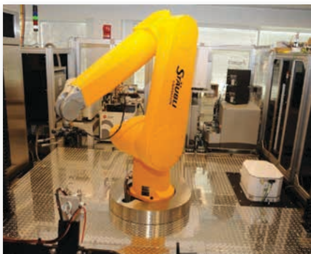
Tox21 robot for high-throughput screening of chemicals for toxic effects
