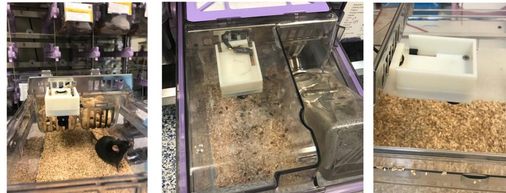
Figure 1: Images of the Cage Cam Mounted in an Allentown NexGen Cage
