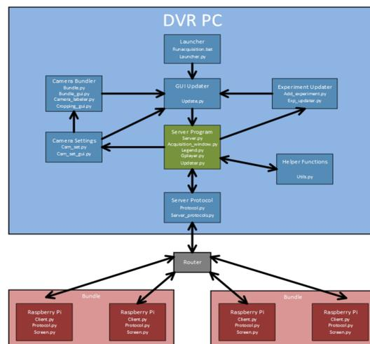
Figure 5. The DVR software model showing the grouping of code files in terms of higher-level function. The diagram shows the code-file to hardware device pairing. In this example diagram, the box labelled DVR PC refers to the computer to which the video is streamed and stored. The example assumes four RPI's each two are bundled as one unit (e.g., two cameras per arena).
