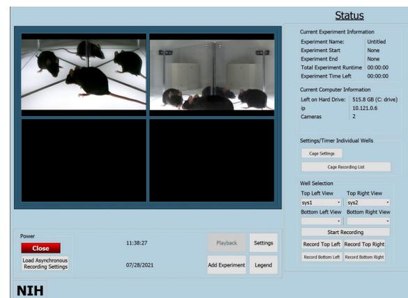
Figure 6: Python based GUI showing two synchronized RPI camera streams. (1 arena being shown)
