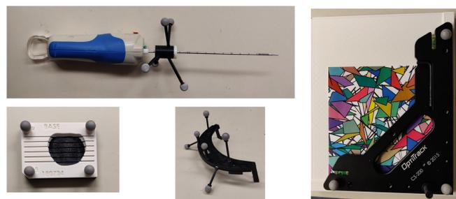
Figure 2. Biopsy needle (top left), prostate mold (bottom left), and HoloLens tracker (bottom middle) with infrared tracking markers, and the calibration square on top of the calibration image (right).
