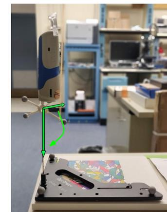
Figure 3. Biopsy needle and markers in the insert with an arbitrary initial orientation and the Y-axis correction.
