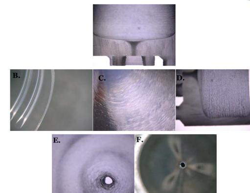
Figure 6. Images of 3D Printed Insert Under a Microscope: A) Image of the pellet well B) Falcon tube surface C) 3D printed insert, glossy finish D) 3D printed surface, matte finish E) Pellet well top view, matte finish F) Pellet well top view, glossy finish
