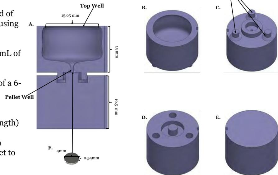
Figure 4. Images of the 3D printed insert parts: A) Assembled, B) Top view of top part, C) Bottom view of top part, D) Top view of bottom part, E) Bottom view of bottom part, and F) Teflon gasket
