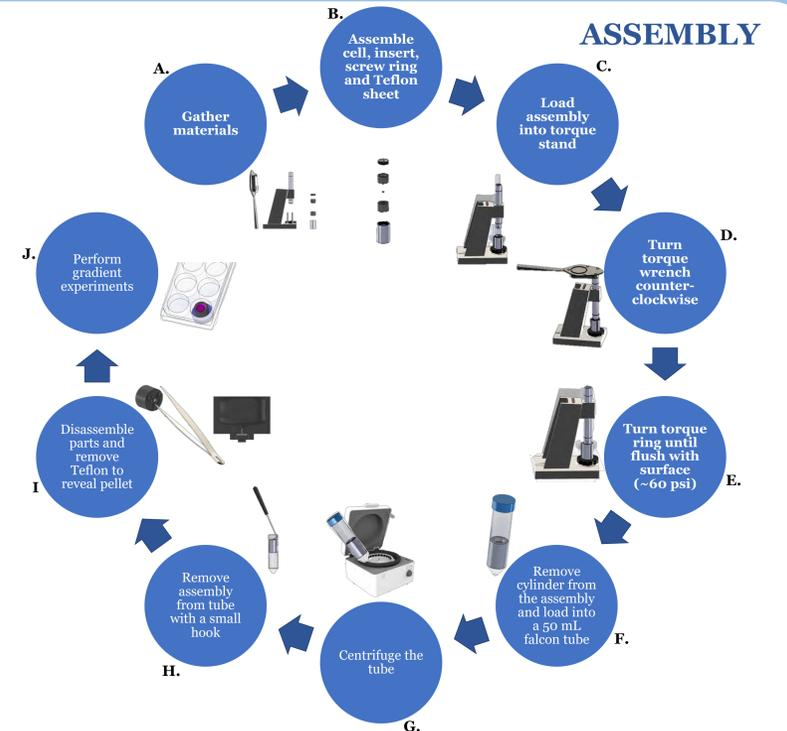
Figure 5. Assay: Insert assembly, centrifuge, pellet, and cell culture gradient experiment.
