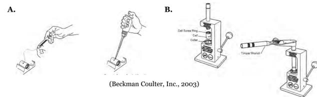
Figure 3. Schematic of analytical ultracentrifugation sample cell preparation: A) Loading sample, and B) Assembly (Beckman Coulter, Inc., 2003)
