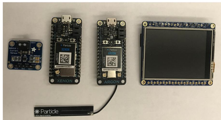
Figure 2: Current monitor, Particle devices, and screen
