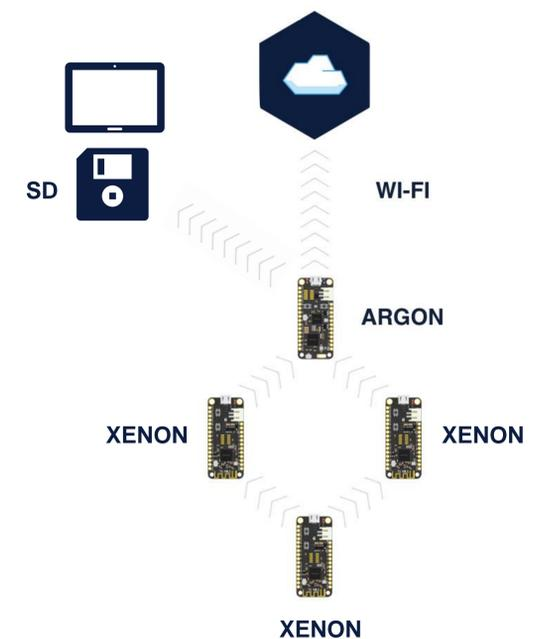
Figure 3: Mesh network diagram
