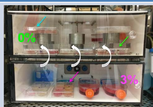
Figure 5. Cells in bioreactor. (A) Anoxic chamber with gradient plate (green arrow). (B) Hypoxic chamber with 3% control plate (pink arrow). (C) Anoxic chamber with 0% control plate (cyan arrow)
