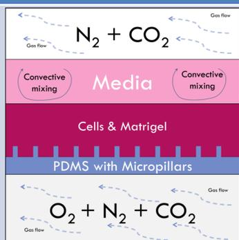
Figure 3. Illustration of PDMS membrane and cell culture material separating the top and bottom chambers.
