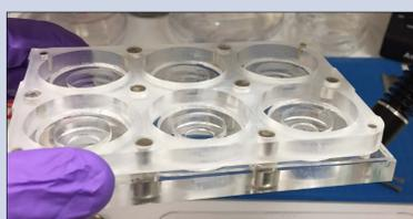
Figure 4. Image of custom 6-well plate with PDMS membrane.
