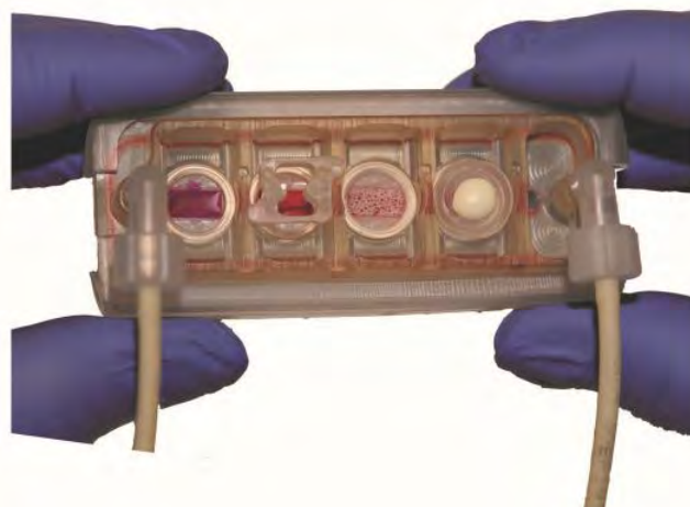
The multi-organ tissue chip system. Types of tissues, from left to right: liver, heart, skin, and bone. Credit: Ronaldson-Bouchard and Vunjak-Novakovic at Columbia University
