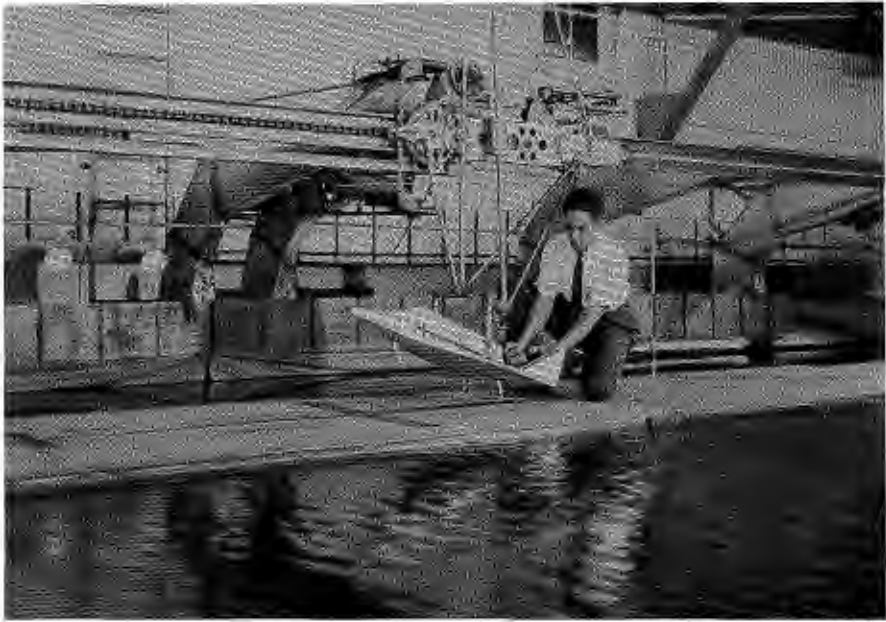
A Langley engineer prepares a model of the proposed air force X-20 Dyna-Soar aerospace plane for testing in Tank No. 2 in 1961.
