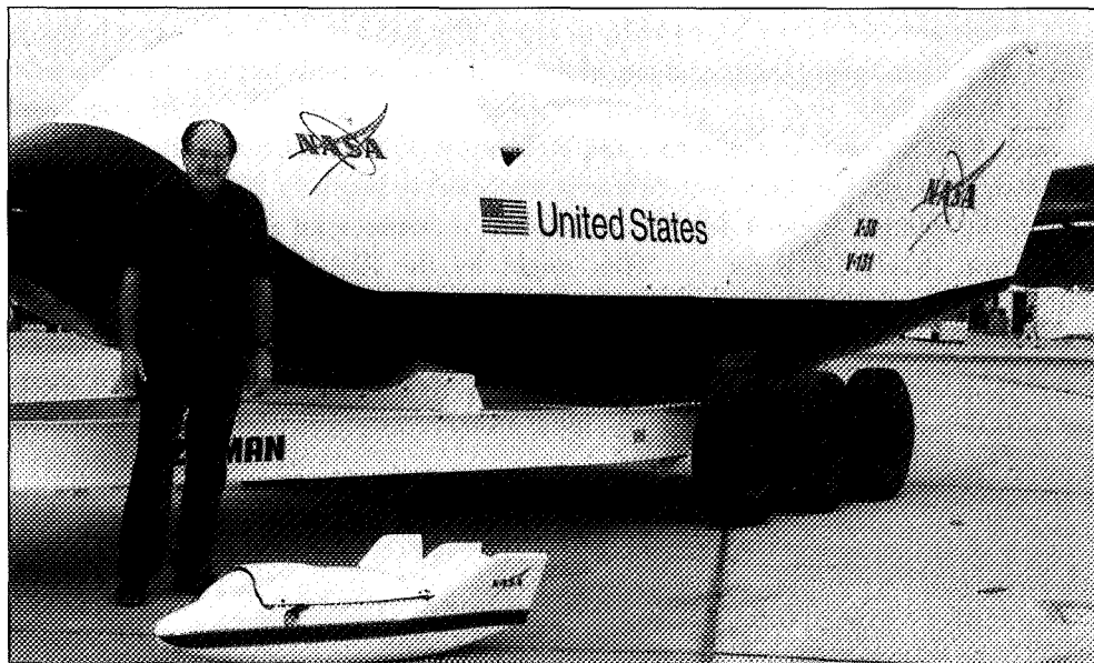
Dale Reed pictured with the X-38 technology demonstrator for a crew return vehicle from the International Space Station and the subscale model used in a test program for the X-38. (NASA photo EC97 44152-5)
