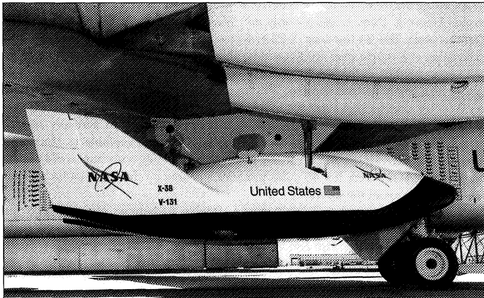
X-38 suspended under the pylon that would attach it to the B-52 mothership for later captive flights and launches. Note that the X-38 has an X-24A shape. (NASA photo EC97 44105-29)
