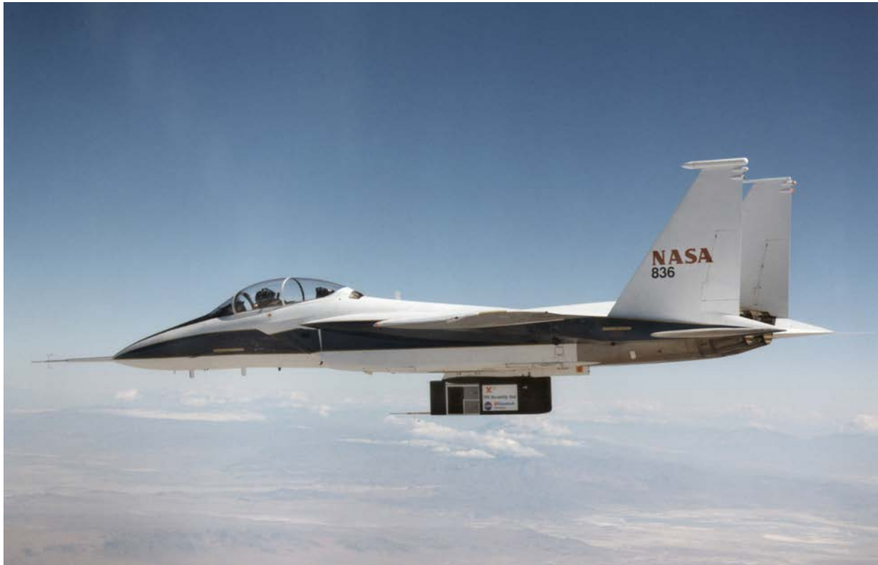
Figure 3-58. Inflight photo of the NASA F-15B used in tests of the X-33's thermal protection system (TPS) materials, 14 May 1998 (NASA-DFRC photo EC98-44554-31).
