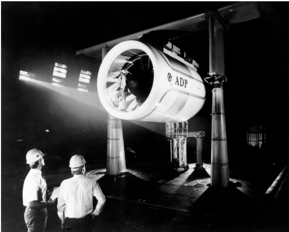
Figure 3-37. NASA engineers are shown preparing a laser light sheet for a flow visualization test of a Pratt & Whitney Advance Ducted Propulsor demonstrator engine in the Ames 40- by 80-foot wind tunnel in 1993 (NASA-HQ-GRIN photo GPN-2000-001521).
