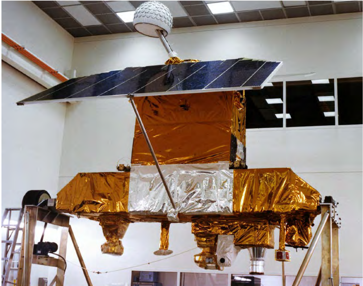
Figure 2-13. The ERBE SAGE II Shuttle Launch Package was designed to measure and analyze fluctuations in the amount of heat energy emitted by the Sun and reflected or absorbed by Earth (NASA photo EL-2001-00409, NASA LaRC).
