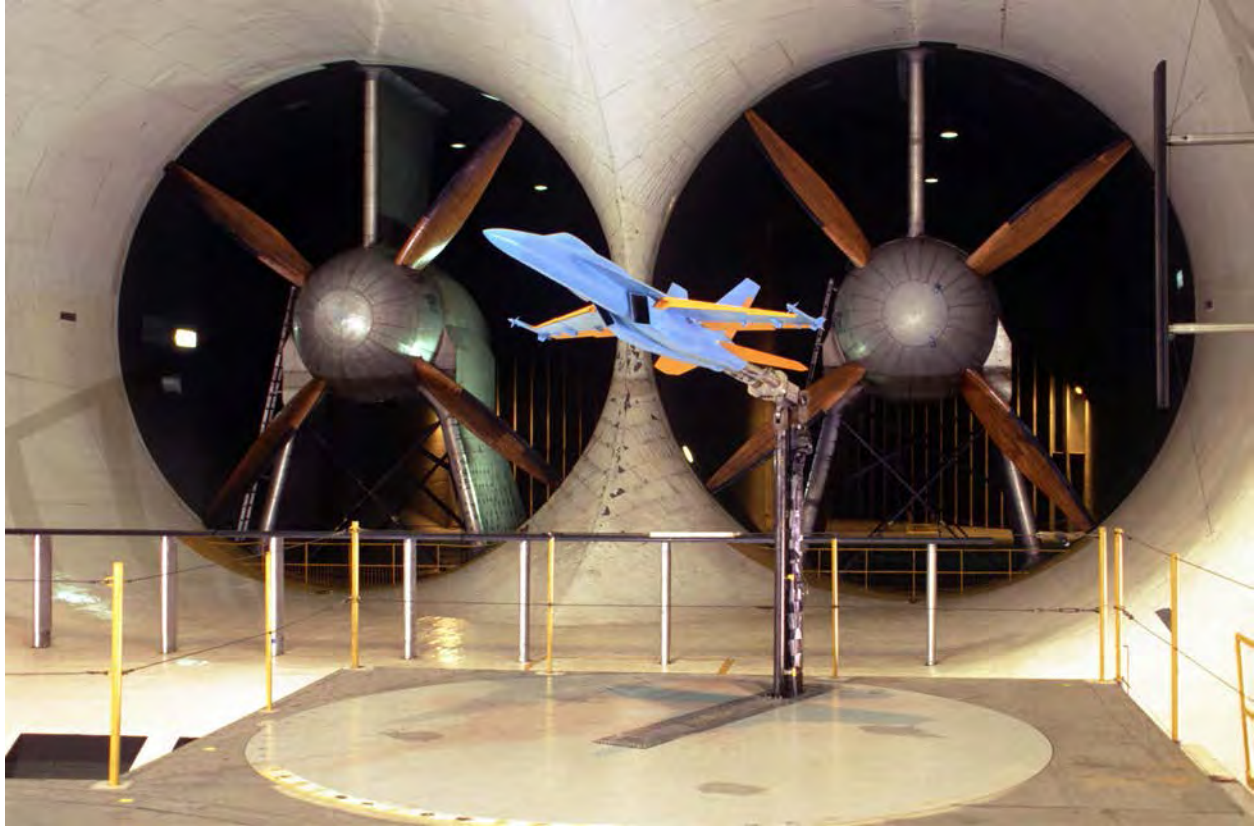
Figure 3-41. The photograph shows a 15 percent scale model of the F/A-18E undergoing low-speed testing in the Langley 30- by 60-foot tunnel (NASA-LaRC photo EL-1996-00196).
