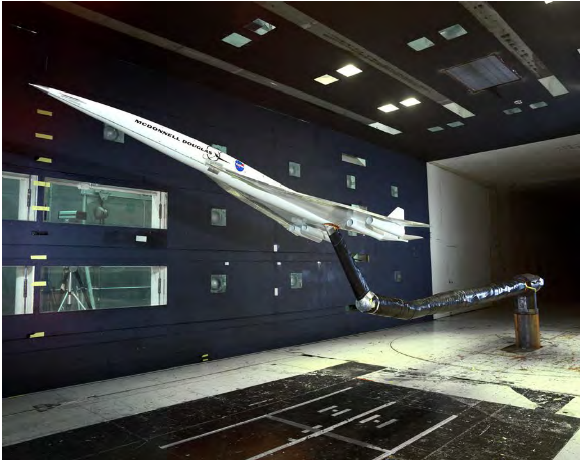
Figure 3-39. A high-speed research model in Langley's 14- by 22-foot subsonic tunnel, 25 August 1995 (NASA-LaRC photo EL-1998-00237).
