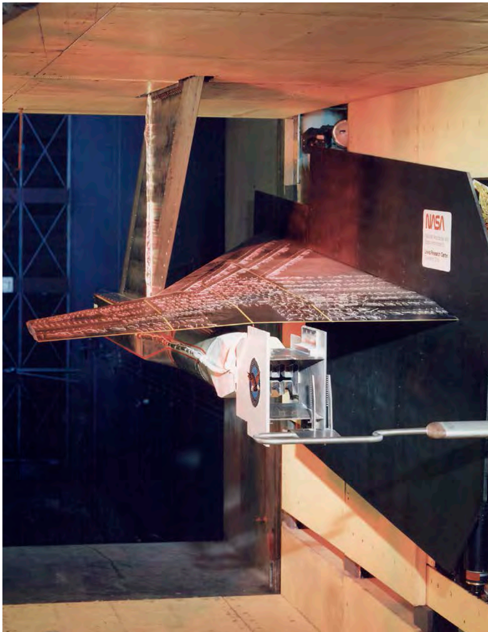
Figure 3-49. This photo shows a nozzle test with a wing section in the 9- by 15-foot wind tunnel (NASA-GRC photo C-1992-205).
