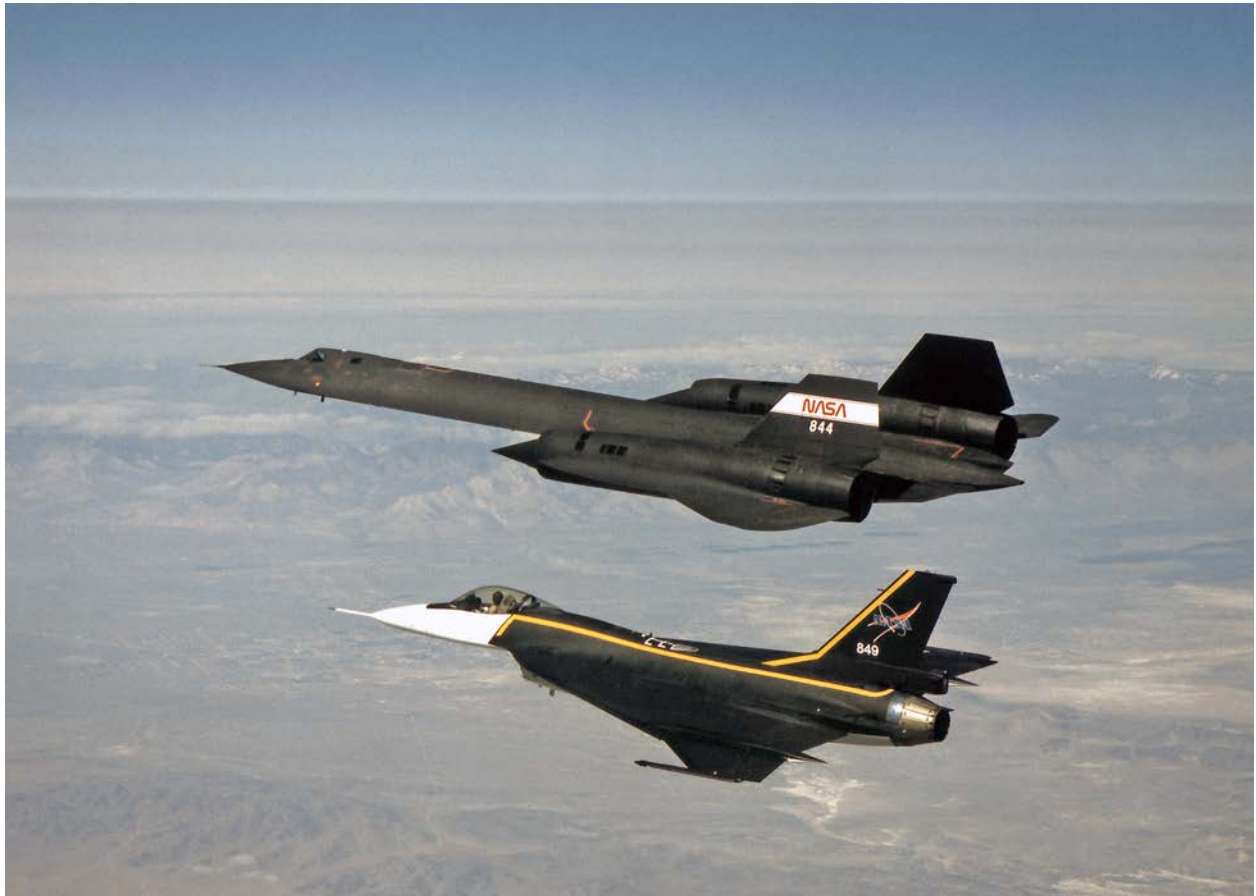
Figure 3-15. The single-seat F-16XL (in the foreground) flies in formation with an SR-71A on one of the flights in the sonic boom research program conducted by Dryden Flight Research Center (NASA-DFRC photo EC95-43024-5).
