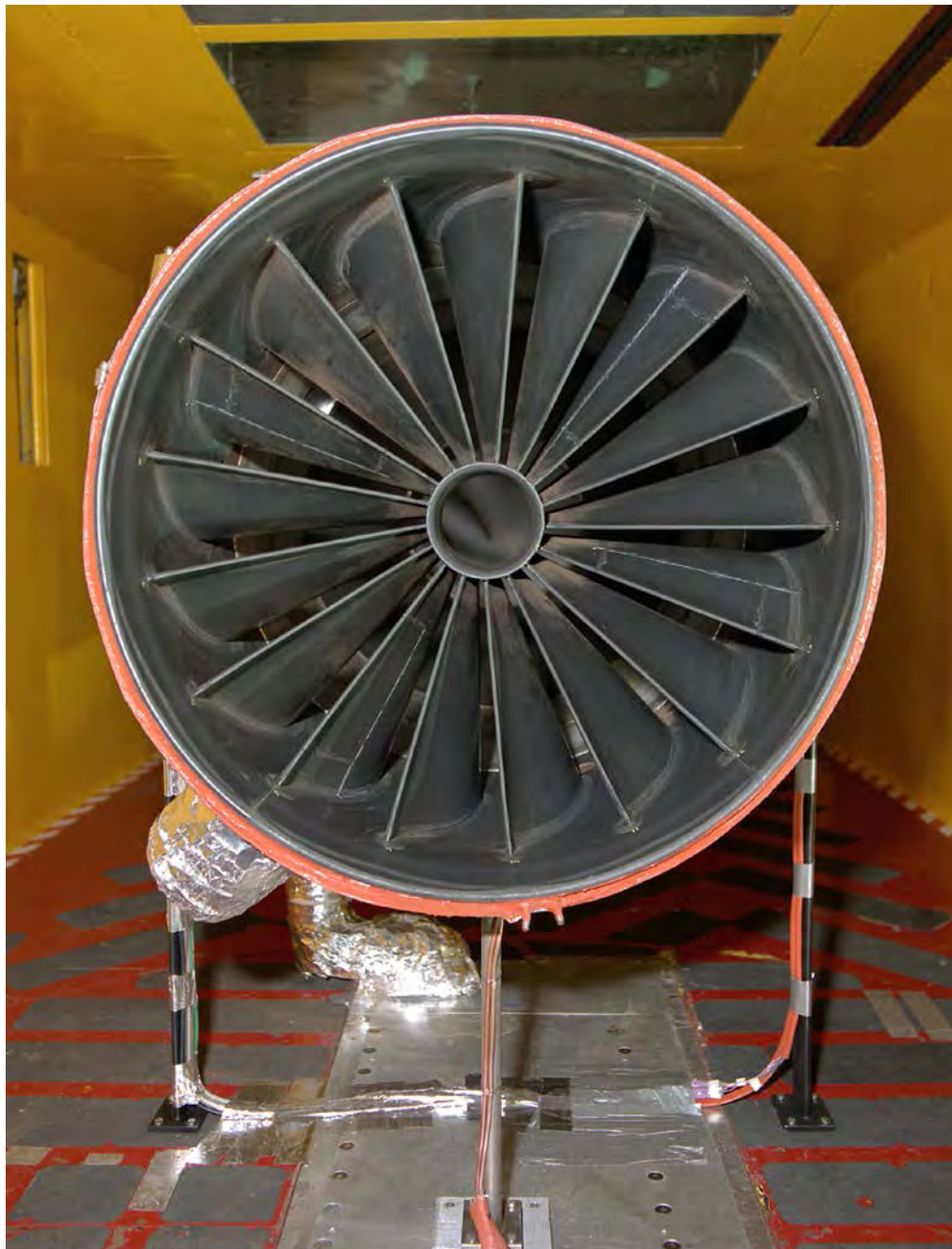
Figure 3-51. F-414 engine in the Icing Research Tunnel (NASA-GRC photo C-1995-1204).
