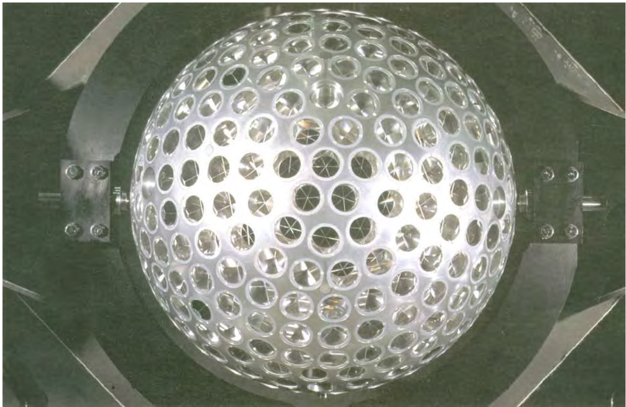
Figure 2-11. LAGEOS II satellite in the apogee stage structure (Alenia Spazio brochure provided by Carey Noll, GSFC).
