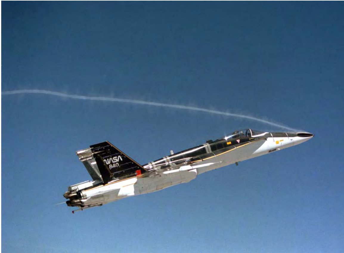
Figure 3-27. This photo shows a smoke-flow visualization of actuated nose strakes with the F-18 High Alpha Research Vehicle (HARV) (NASA-DFRC photo EC96-43479-5).
