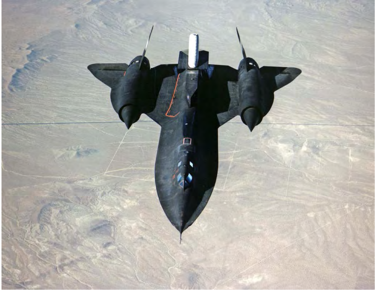
Figure 3-28. 10A NASA SR-71 made its first successful flight 31 October 1997 as part of the NASA/Rocketdyne/Lockheed Martin Linear Aerospike SR-71 Experiment (LASRE) at Dryden Flight Research Center (NASA-DFRC photo EC97-44295-51).
