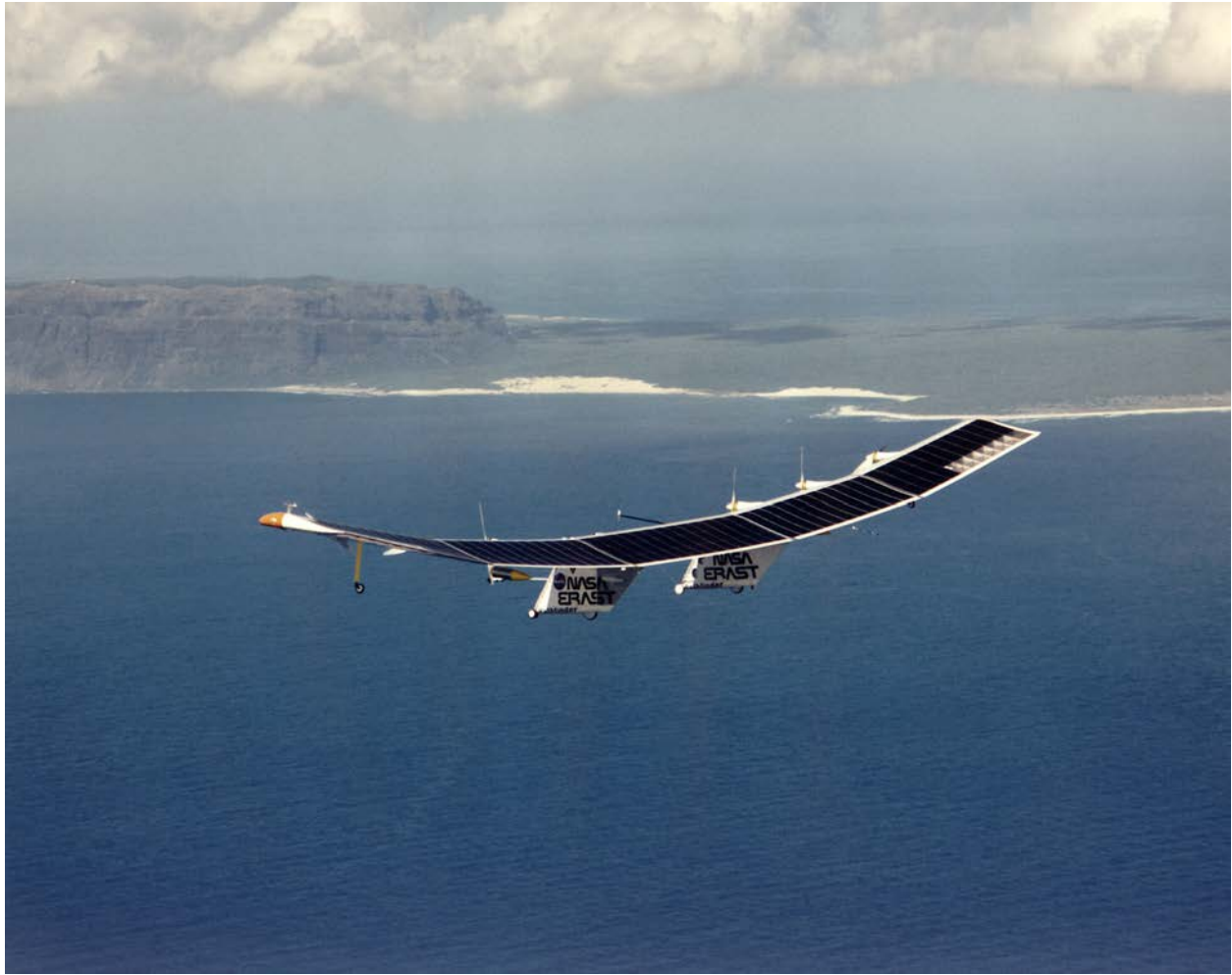
Figure 3-20. Pathfinder, NASA's solar-powered, remotely piloted aircraft, is shown while conducting a series of science flights in August 1997 in which it collected imagery of forest and coastal zone ecosystems on Kaua'i, Hawaii (NASA-DFRC photo EC97-44287-2).
