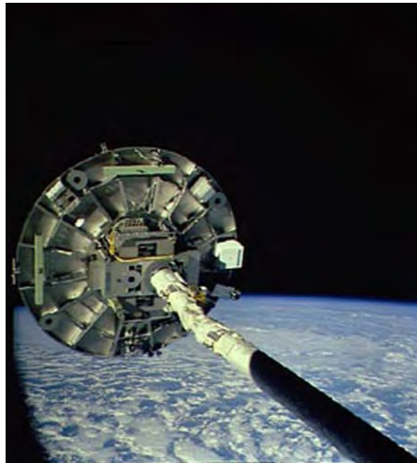
Figure 2-39. The Wake Shield Facility (WSF), pictured at the end of the Shuttle's robot arm, is a free-flying research and development facility that uses the pure vacuum of space to conduct scientific research on the development of new materials. The thin-film materials technology developed by the WSF could some day lead to applications such as faster electronics components for computers (NASA photo MSFC-9901881).
