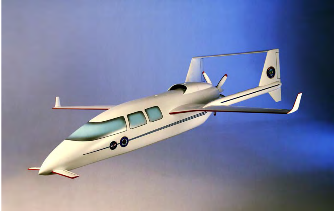
Figure 3-14. This photo illustrates an AGATE advanced concept airplane. The pusher propeller-driven configuration seats four to six people (including the pilot) in a midwing, three-surface, twin-tailboom configuration. The design concept incorporates natural laminar flow, ice protection, winglets, and stall-departure-resistant flight dynamics (NASA LaRC photo EL-1996-00214).
