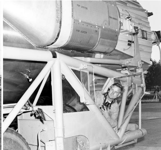
*Image 80: General Dynamics designed a unique 64-foot-long cradlelike trailer to transport the missile. It was so large that additional drivers were placed at the rear of the trailer to guide it around turns (GRC-1963-P-01708).<sup>351</sup>*
