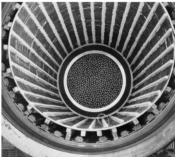
*Image 219: Pellets inside HHTF's pebble bed heater (GRC-1966-P-01889).*
