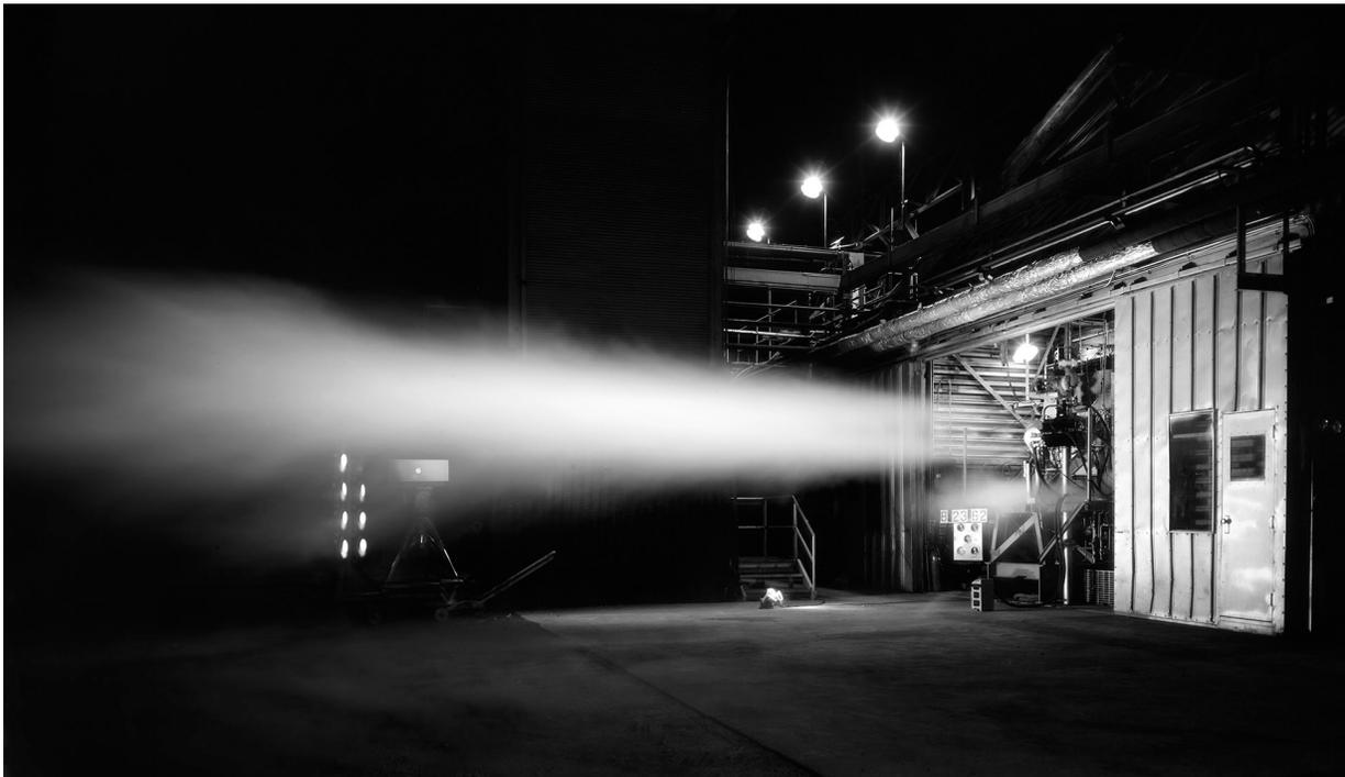
*Image 74: Firing of the copper nozzle rocket with gaseous hydrogen and liquid oxygen at J-1 in 1962 (GRC-2016-C-05089).*
