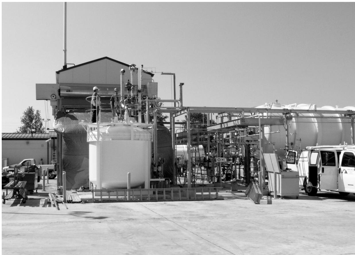
*Image 180: Cryogenics Components Lab at Plum Brook. The complex includes test cells (some of which were moved from Lewis Field) to study liquid oxygen, nitrogen, and hydrogen; a hydrogen densification area; and an area for the high-pressure testing of tanks (GRC-2004-C-01205).*
