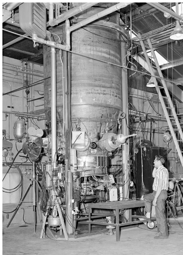
Image 115: Boiling Fluids Rig inside of C Site (GRC-1961-C-57350).
