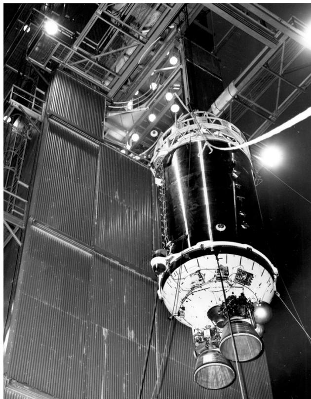
*Image 75: A Centaur stage is lifted into E Stand just before dawn in January 1964. Centaur was powered by two Pratt & Whitney RL-10 engines, which ran on liquid hydrogen and liquid oxygen (GRC-1964-P-01084).*
