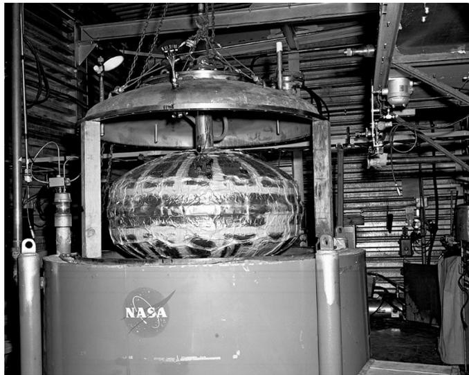
*Image 89: Linde superinsulated tank at the J-3 facility in May 1963. The 150-gallon stainless steel tank was designed to be suspended by its neck, so it was not a true space tank (GRC-1963-P-01446).*
