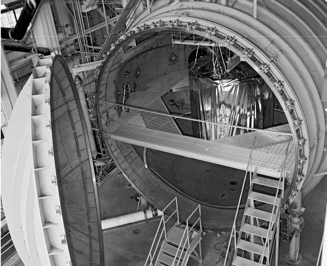
*Image 130: K Site test chamber with cryoshroud installed around the tank. The cryoshroud, or cold wall, subjected the tank to the low temperatures encountered in space (GRC-1971-P-01399).*
