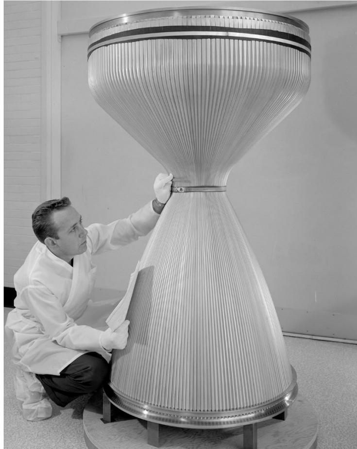
*Image 105: A Lewis engineer examines the cooling passages on a converging-diverging nozzle for a nuclear engine. The nozzle had a unique 12 to 20 contraction ratio and 45-degree contraction half-angles<sup>450</sup> (GRC-1963-C-66545).*
