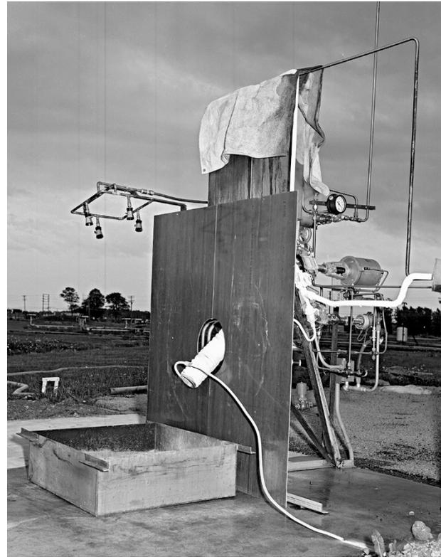
Image 120: Photo of the spill test setup near J-5. A vertical aluminum shield was placed between the pan and the stand to protect the latter from damage<sup>521</sup> (GRC-1964-P-91511).
