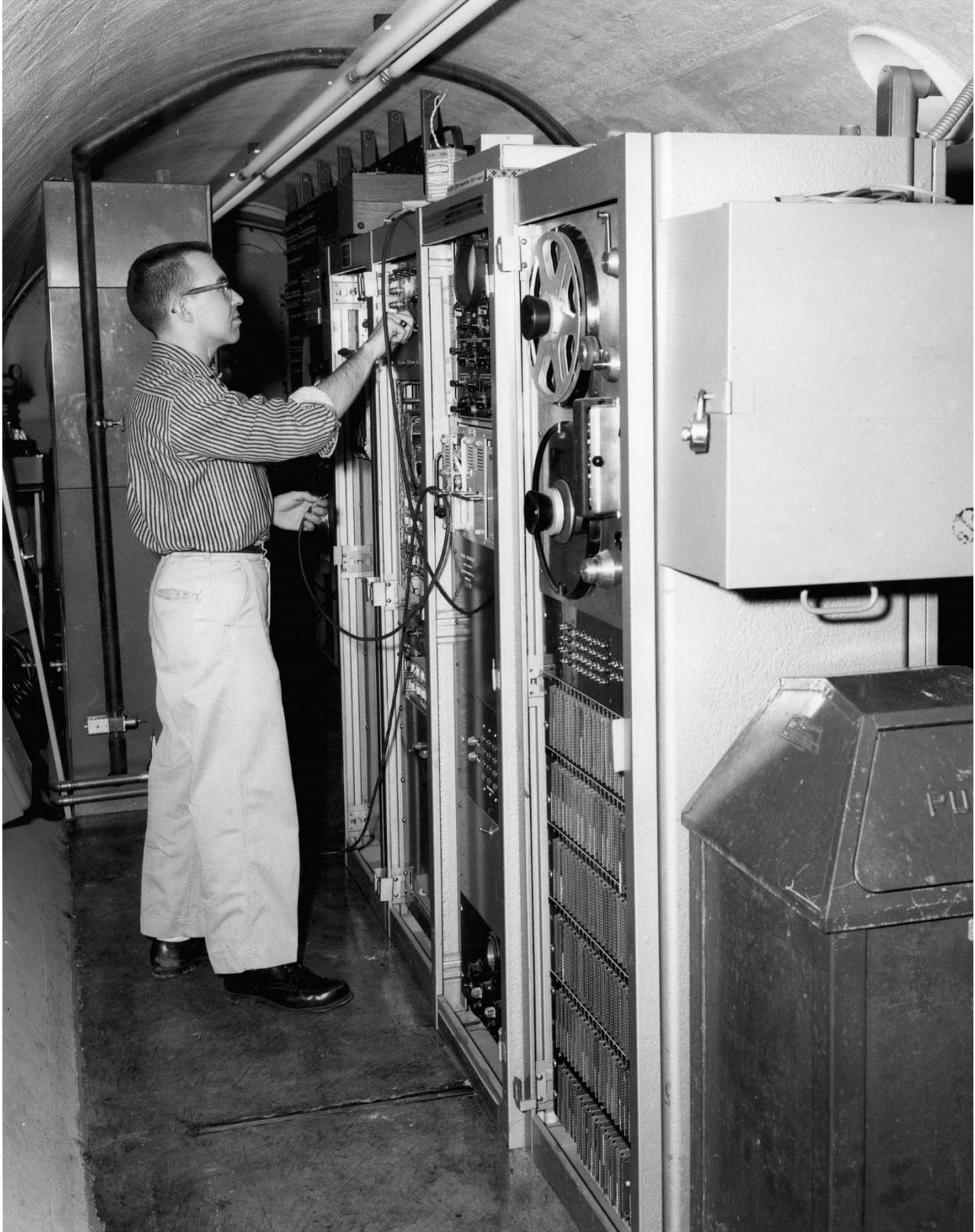
*Image 42: An operator inside the control room for the Pilot Plant. The control room was built inside a 9- by 36-foot tubular PBOW tank (GRC-2016-C-05167).*
