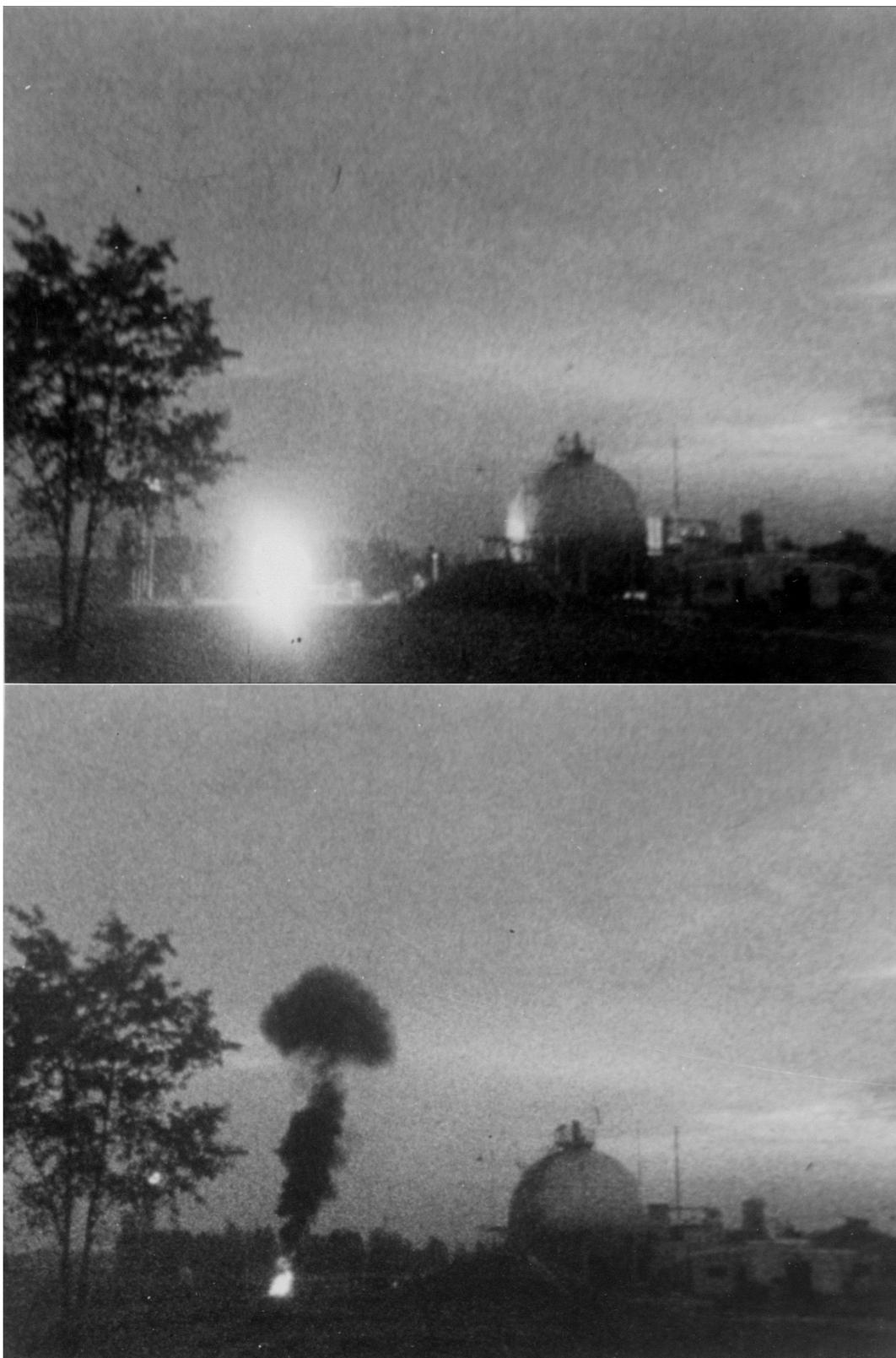
*Image 118: Top: Fireball from FLOX spill onto JP-4 fuel. Bottom: Resulting fire 2.5 seconds later on 6 October 1965 (GRC-1965-C-02830).*
