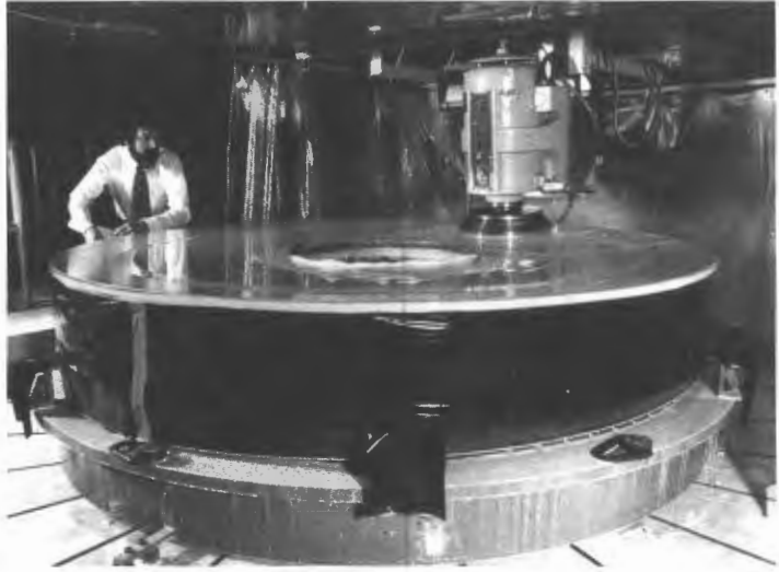
Initial polishing of space telescope primary mirror blank at Perkin-Elmer, Danbury, Connecticut, May 1979.
