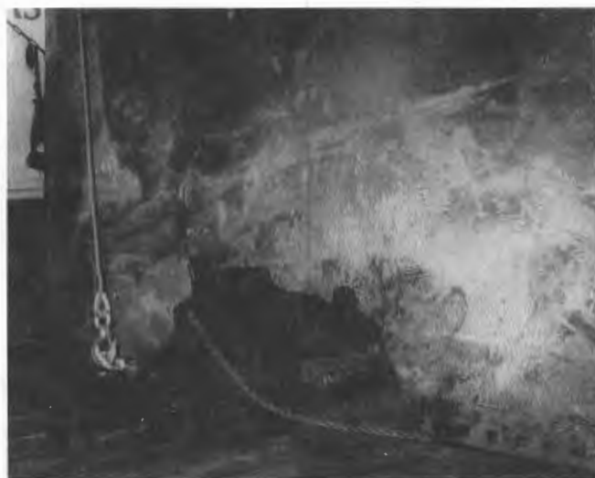
Photo of recovered fragment of aft center segment of right SRM of STS 51-L, showing hole burned through the case wall.
