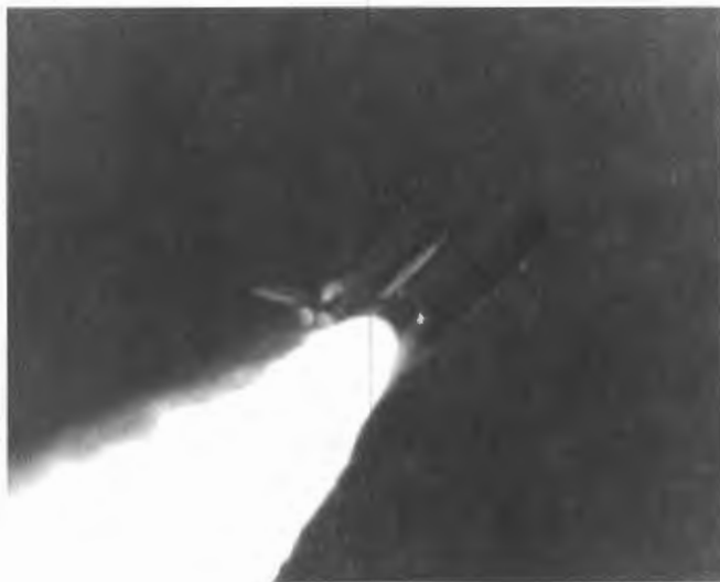
Plume of flame from aft field joint of right SRM of STS 51-L, approximately 60 seconds after ignition.
