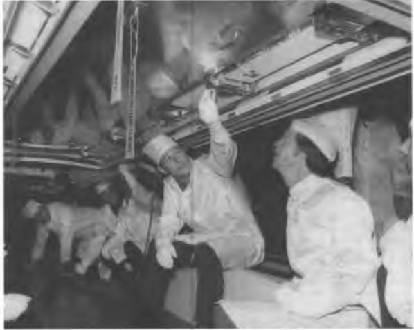
Testing the twin-pole sunshade at the Skylab mock-up in Building 4619.
