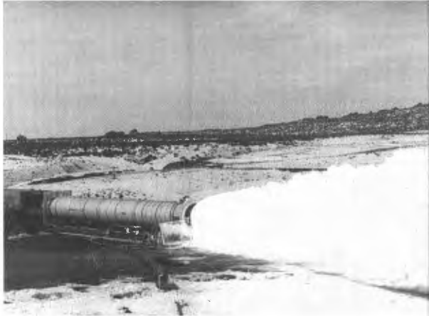
Static firing of the solid rocket motor in northern Utah in February 1979.
