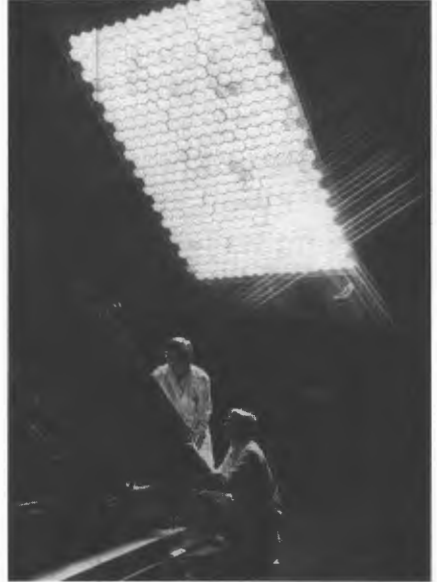
Test of a solar collector in simulated sunshine at the Marshall Center, 1978.
