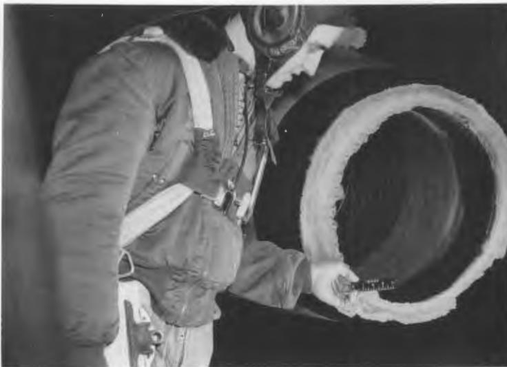
*A NACA pilot measures ice on a turbojet engine's inlet. Until 1950 flight into icing clouds provided more reliable data than tests in the Icing Research Tunnel.*
