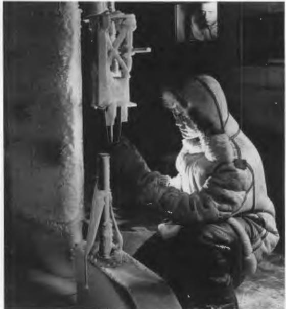
*Two instruments to measure icing rates during flight through an icing cloud are calibrated in the Icing Research Tunnel. The lower device is Langmuir's rotating multi-cylinder. The upper u-tube device is the NACA pressure-type icing meter used to gather statistics on the duration and severity of icing encounters in the early 1950s.*
