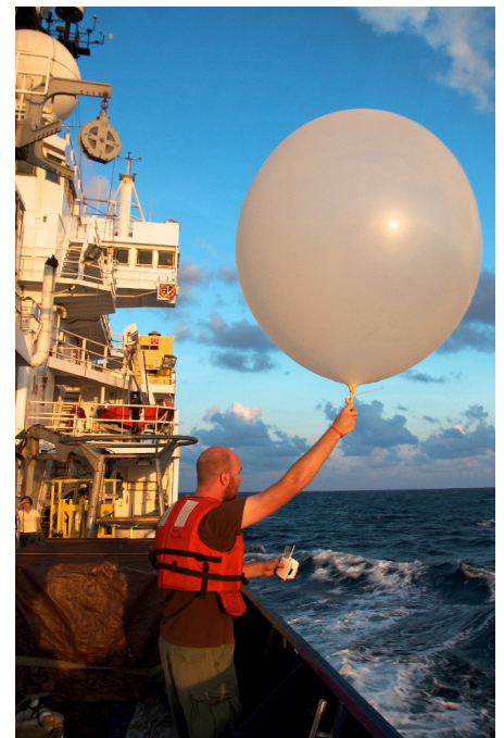
A researcher launches a radiosonde instrument attached to a weather balloon to capture detailed atmospheric data. Credit: National Center for Atmospheric Research.
