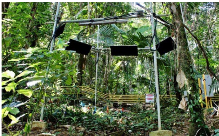
A warmed TRACE plot in the USDA-Forest Service Luquillo Experimental Forest in Puerto Rico. Three 15-foot diameter areas are warmed 7°F above surrounding temperatures with an array of six infrared heaters; three areas of the same size receive the same infrastructure but are not warmed. Source: Tana E. Wood, USDA.
